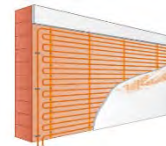
Plastered wall heating/cooling
