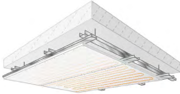
The ModuleCeiling-Classic for non suspended ceilings
