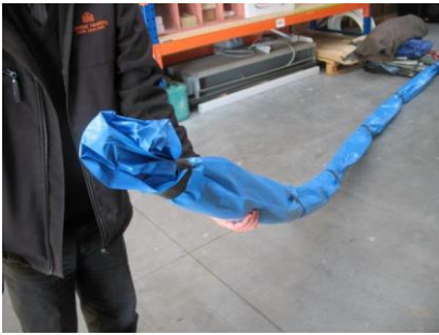
Pipe sleeved in waterproof bagging and sealed at both ends.
