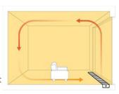
to the glazed façade. This can prevent the formation of condensation on the windows and reduce the radiant cooling effect on those inside, improving the comfort and functionality of the building.
