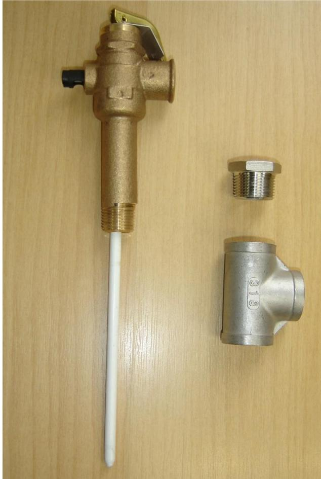
Reliance 850kPa, 99°C TPR kit supplied with the 200 and 300 litre single coil cylinders. May need to fitted before siting the cylinder if headroom is limited.
