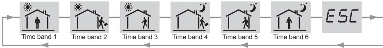
The time bands on systems with multiple zones, each of which is managed by its own room controller (maximum 6), must be programmed on each room controller.
