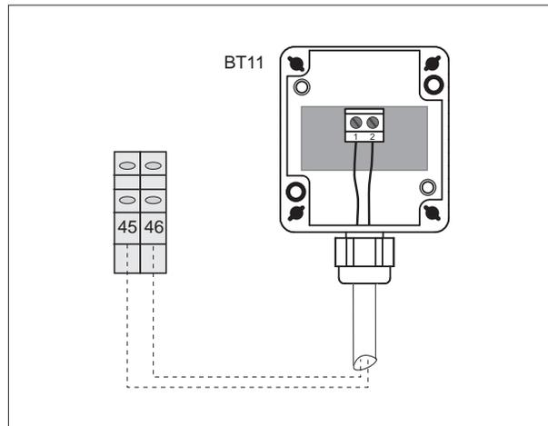
**Water outlet and return temperature probe BT1 and BT2 connection to heat pump**
