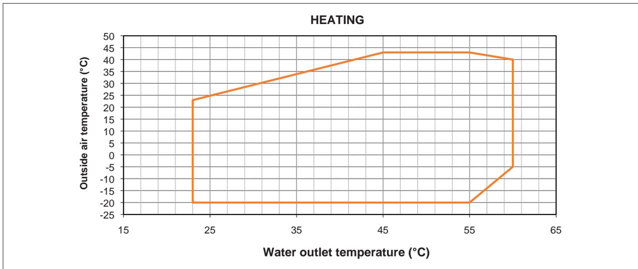
Min/max water temperature difference = 5/10 °C (in minimum flow conditions, 7 l/min)
