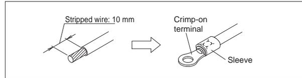
(3) Use the cables specified, connect them securely and in such a way that they don't exert pressure on the terminals.
