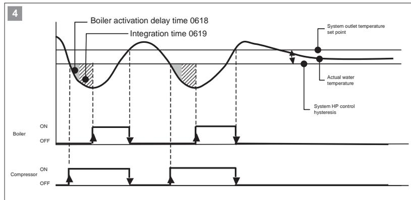
Once the boiler has been enabled, supplementary heating is activated when the integration time set for parameter 0619 is reached and the delay time 0618 has elapsed. The delay time is ignored when the unit is first started.
