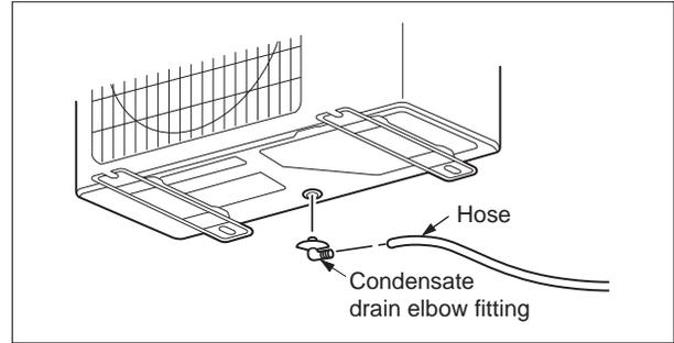
If the outside air temperature is less than 0°C, the condensate drained from the collection pan may freeze.
