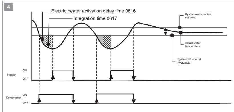
Once the heater is enabled, supplementary heating is activated when the integration time set for parameter 0617 is reached and the delay time 0616 has elapsed. The delay time is ignored when the unit is first started.
