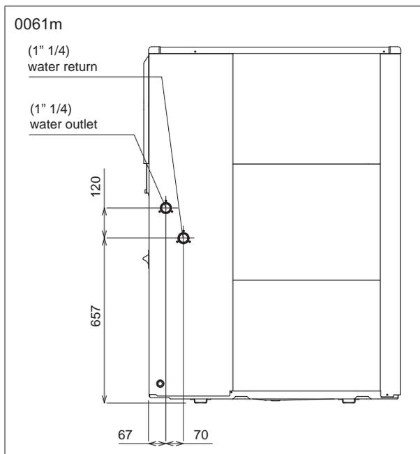
Construction of a bypass is recommended to enable the pipes to be washed through without having to disconnect the unit (see drain valves). The connection piping should be supported in such a way as to avoid it weighing on the unit.
