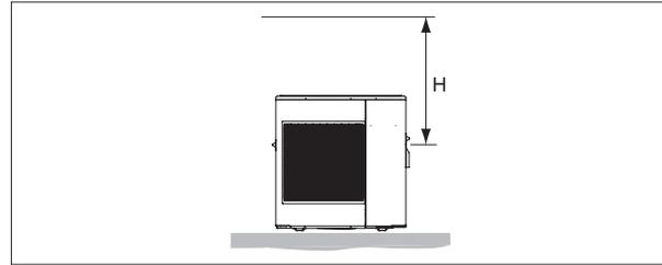
For height differences exceeding 12 metres, the volume of water in the system as described above may decrease; evaluate whether the expansion vessel supplied is sufficient for each system, otherwise install an additional expansion vessel.
