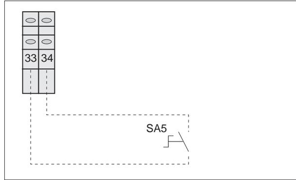
Contact closed: forced operation during the reduced rate period.
